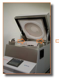
By ordering the **prepASH®** with the option ECD, the system will be equipped with two fans to deliver air with ambient temperature to the sample room.
