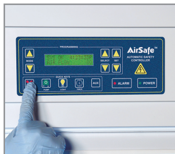
Real-time monitoring of face velocity and filter condition via AirSafe
