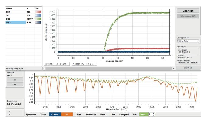
OPUS GA user interface: The time series window (top) displays the concentration of selected gas compounds as a function of time. In the Spectral Analysis window (bottom), the measured spectra can be investigated in detail. The measured spectrum (blue), the fit (orange) and the contribution of the target gas  $N_2O$  (green) to the overall spectrum are shown in a selected spectral region. An excellent agreement between measured spectrum and fit is obtained.
