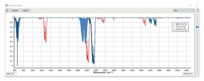
The simulation tool can be used to visualize IR spectra of gas mixtures in order to define or modify quantification methods. The spectra of all compounds that are part of the spectral database (more than 350) can be simulated considering concentration, temperature, pressure and spectral resolution.
